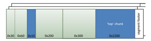
When you call free on a given chunk, the first thing that happens is that dlmalloc checks to see if the preceding chunk is in use. If the preceding chunk is free, dlmalloc will consolidate the two chunks into one larger free chunk.
