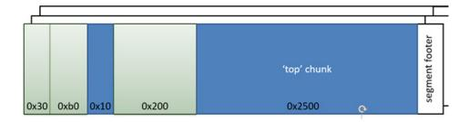
When dimalloc needs to allocate a new chunk for a malloc call, it will check if the top chunk is big enough to contain the new chunk, and will carve the new chunk from within the top chunk by splitting it. The first half of the top chunk becomes the new chunk to be returned, and the second half becomes the new 'top chunk'. If the 'top chunk' is not large enough to contain the new chunk, a new segment is allocated from the operating system, and the new chunk is allocated from that new segment.
