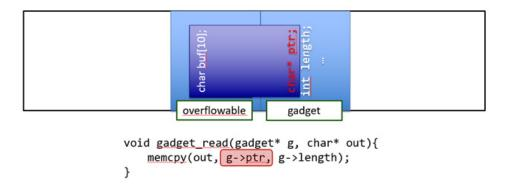
We can then cause the overflow, overwriting the pointer in the gadget object's data structure with a pointer of our choice. We then trigger the read operation to read data at our desired pointer.
