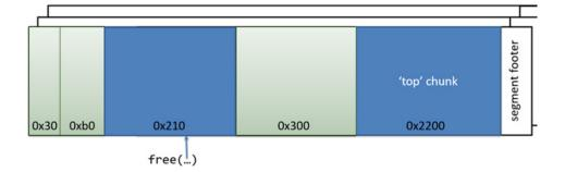
This means that it is impossible for two consecutive chunks in a segment to both be free. The chunks immediately before and after a free chunk are both guaranteed to be in use.
