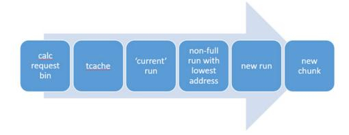
So when allocating on jemalloc, we observe the following flow.
