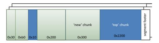
Each chunk has two pointers worth of metadata: in 32bit processes this is 8 bytes. This metadata sits directly before the pointer returned by malloc, i.e. inline before the useable memory. The minimum amount of actual usable memory returned by malloc is two pointers wide.
