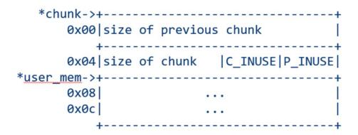
Chunks of different sizes can be allocated one after the other in the segments. Each chunk marks its size and whether it is in use or not, via the C\_INUSE flag. It also marks whether the previous chunk in the segment is in use, with the P\_INUSE flag, and the previous chunk's size. Because the metadata contains the size of the previous chunk, we can easily walk backwards through the chunks in a segment.
