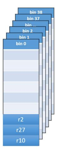
Regions which are currently held in tcaches do not have their in-use bit set to free. Instead they are considered by the greater jemalloc system to be in-use. This saves on locks, as it is only necessary to grab a lock when updating global data structures. Thread specific data structures are by definition safe from other threads, and thus in many cases jemalloc allocations will not grab locks at all.
