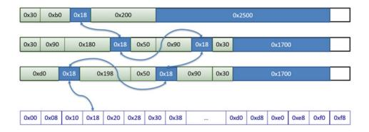
Here's an example showing a few segments with some in use and free chunks. The 0x18 bin points to the first of the free chunks of size 0x18, and the rest of them are chained together in a doubly-linked-list.
