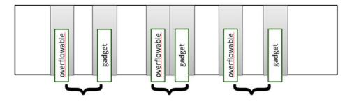
The idea is simple. Using our arbitrary allocation primitive, we allocate a bunch of placeholder sets for our target objects, at the sizes of those objects. Each set of placeholders has a placeholder for the overflowable object and a placeholder for the gadget object. We hope that at least one set of placeholders is allocated such that the overflowable placeholder is directly before the gadget placeholder.
