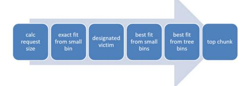
So for a small allocation, a request size smaller than 0x100 bytes, this is the flow:
